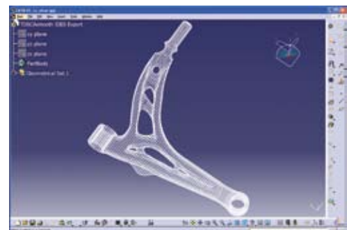
Creation of slices and cutting splines for CAD import of the wishbone illustrated in the title workflow (Images courtesy of Otto Fuchs KG)
