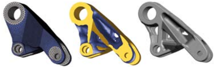
Topology optimization of a tractor lever using TOSCA Structure.topology with casting restrictions leads to a clear rib layout (Images courtesy of JCB)
