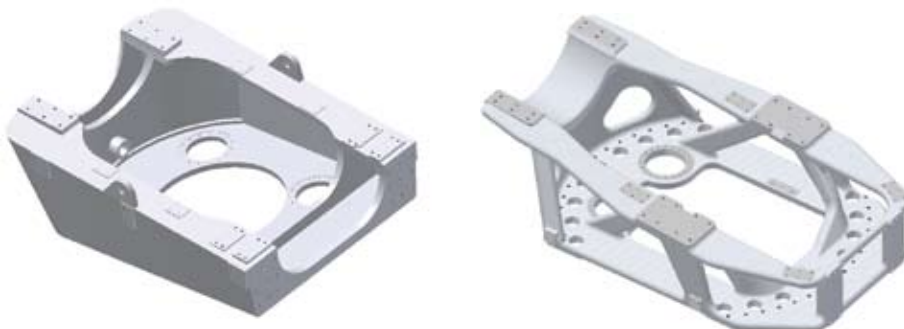
Topology optimization leads to 25% mass reduction with the new design
