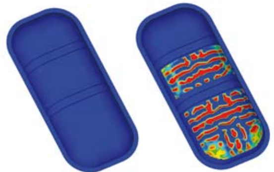
By bead optimization the eigenfrequencies of an exhaust muffler are increased (Images courtesy of Tenneco Automotive)
