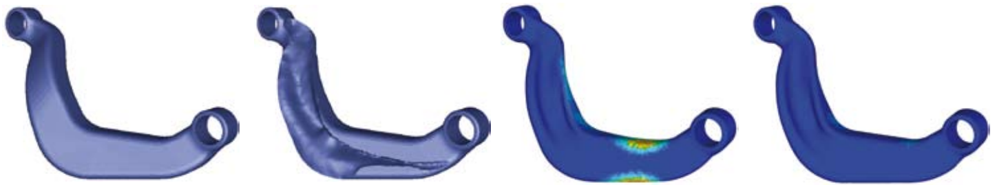
Complete design cycle of topology and shape optimization of a control arm with manufacturing restrictions for forged components
