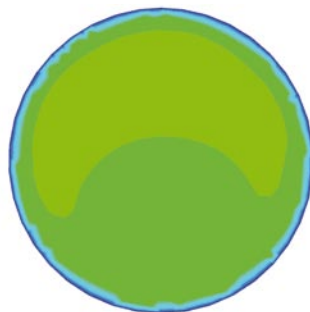
Flow velocity Profile at outlet cross section area for the optimized 180-degree bend
